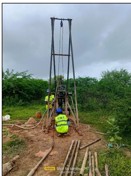
Photo 40 & 41: Calyx rotary drilling machine used for drilling in Reldi Moti Area, Kachchh District, Gujarat
