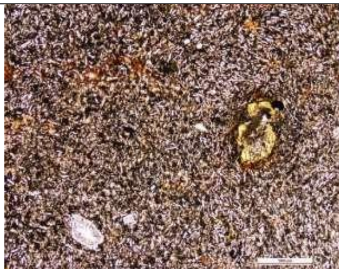
Photo 10: Fine grained basaltic rock with very few zeolites and phenocrysts
